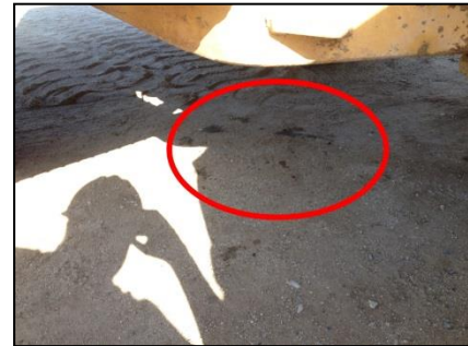
Leaking fuels are a common source of pollutants within vehicle storage areas.
