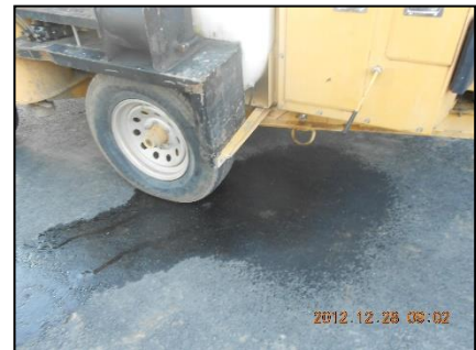
Clean leaks like this using a damp mop or absorbent cloth. Do not hose down.
