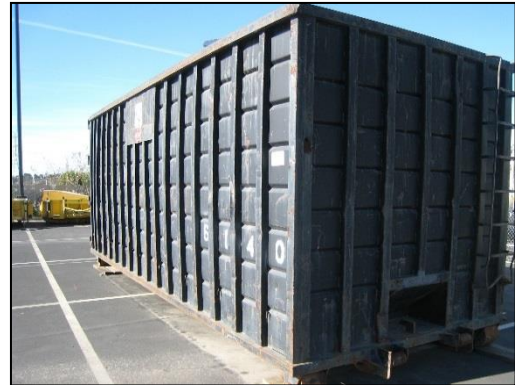
Solid waste receptacles such as this one are effective at preventing contact with stormwater runoff.
