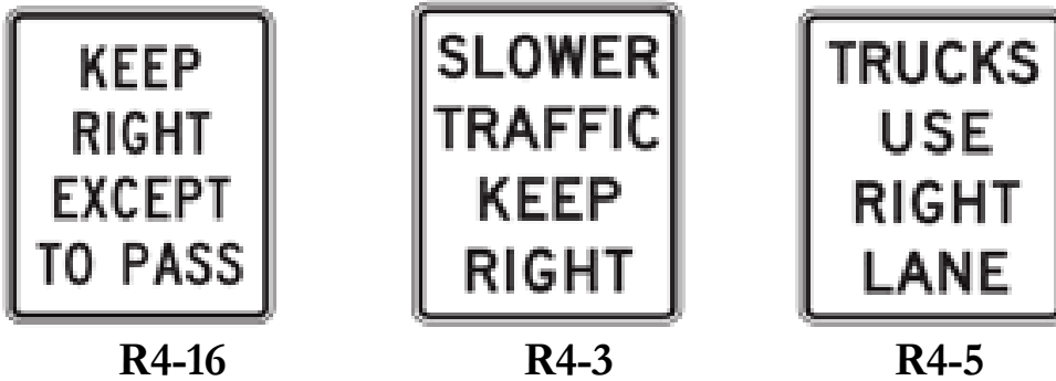
Figure 2 – Regulatory Signs (MUTCD, Figure 2B-10)
