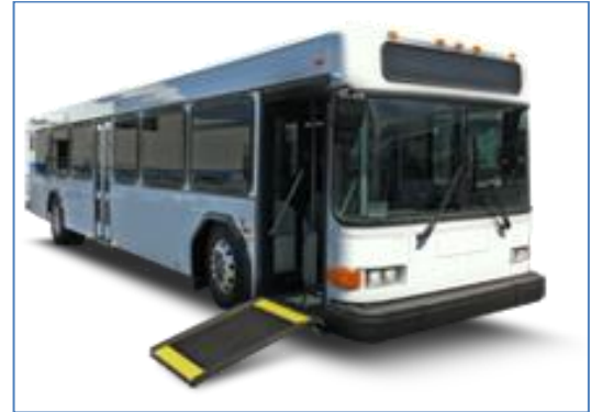
Figure 5-3: Low Floor Bus
